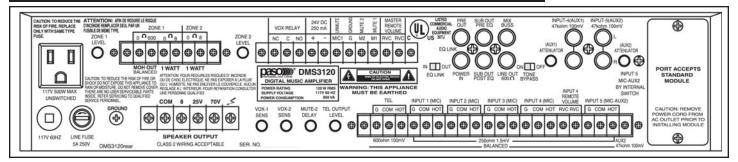
**Inputs 1 - 5 -** Inputs 1 - 5 are set as Microphone Inputs.Impedance is 250 ohm balanced. Input 4 can be switched to AUX 1, Input 5 can be switched to AUX 2 (internal jumper). Impedance is 47 K ohm.
