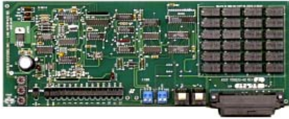
OV-LIB3 12-Line Relay Board (for use with the 'Ovation' Lobby Entry Master Station or with DPW100W Concierge Phone)
